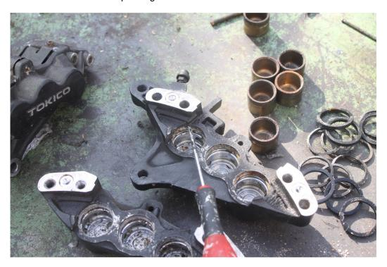
This stops the piston moving outward [finding it's new position] as the pads wear causing excessive brake lever travel.
